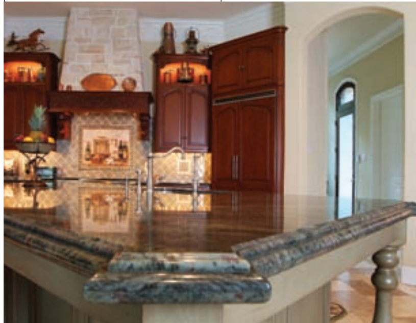
ABOVE: The decorative diagonal corners of the kitchen island designed by Kirk Craig and fabricated by ICM Marble & Granite meant the granite had to be placed atop the base very carefully. The 700-pound countertop required six ICM workers to lift and set it in place.
